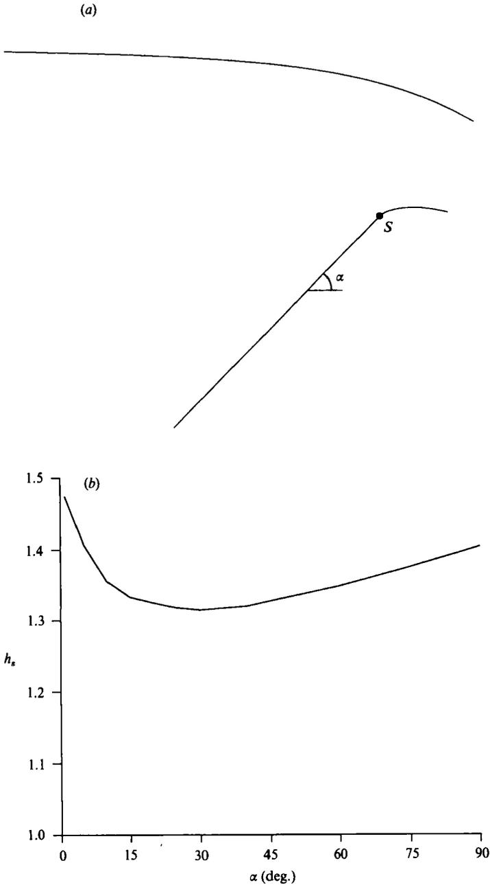
FIGURE 6. (a) Liquid flowing over an inclined weir. Computed solution for  $\alpha = 45^\circ$ . (b) Plot of the elevation of the free surface relative to the elevation of the top of the weir as a function of the angle of inclination of the weir.
