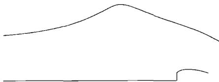
FIGURE 11. Computed supercritical flow of 'solitary-wave-type' for  $F = 1.27$  and  $t_c = 0.375$ . The corresponding value of  $w$  is 0.17. The horizontal scale is the same as the vertical scale.
