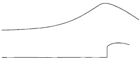
FIGURE 12. Computed supercritical flow of 'solitary-wave-type' for  $F = 1.46$  and  $t_c = 0.2$ . The corresponding value of  $w$  is 0.37.
