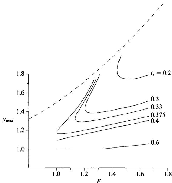
FIGURE 10. Plot of  $y_{\max}$  versus  $F$  for certain values of  $t_c$ .  $y_{\max}$  is the elevation of the highest point on the upper free surface. The short-dashed curve represents the maximum elevation  $y_{\text{stag}}$  that the free surface can ever reach (see (5)).
