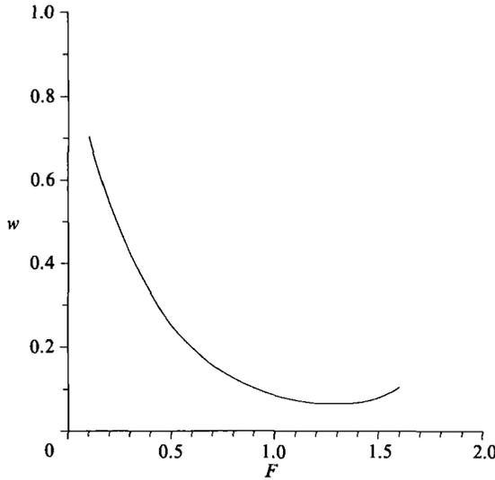
FIGURE 5. Plot of the dimensionless height of the weir  $w$  as a function of the Froude number.
