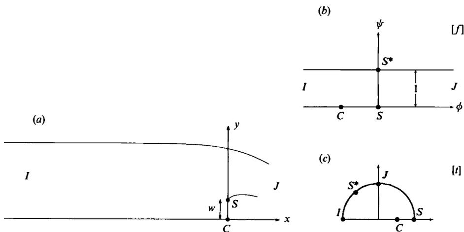
FIGURE 1. (a) Liquid flowing over a thin weir. The flow shown here was calculated for  $F = 0.5$ .  $S$  is the detachment point. The dimensionless elevation of the free surface far upstream is 1. The resulting  $t_c$  is 0.12 and  $w = 0.25$ . The horizontal scale is the same as the vertical scale. (b) Plane of the complex potential. The dimensionless height of the strip is 1. (c) Intermediate plane ( $[t]$ -plane).
