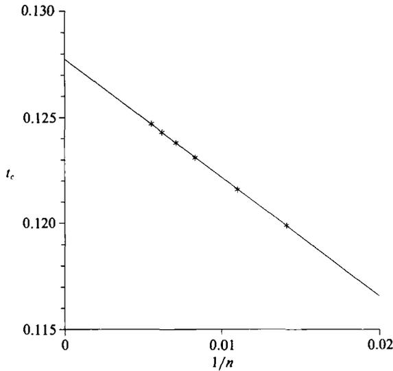
FIGURE 2. Output  $t_c$  for subcritical weir flows as a function of the number  $n$  of collocation points into which the free surface is discretized. The Froude number is 0.5.
