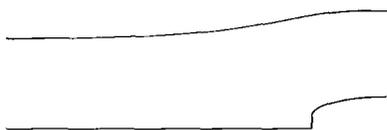
FIGURE 13. Computed supercritical flow of 'waterfall-type' for  $F = 1.66$  and  $t_c = 0.4$ . The corresponding value of  $w$  is 0.16.
